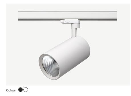
For use in retail, commercial, and residential accent lighting applications, designed for the illumination of merchandise or artwork. T55 is track mounted miniature LED spotlight fixture with integral driver. Offered in 3000K with a CRI of 90-plus, the fixtures are available in Max36W. Beam spread options include 15 degree, 24 degree, and 36 degree. Fixtures are available in white, black.
